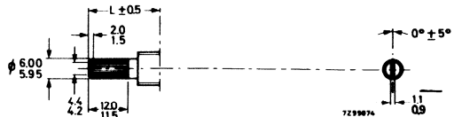
Fig. 3. Spindles in fully counter clockwise position ("off" position)
