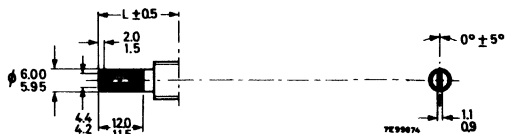
Fig. 3. Plastic spindles in fully counter clockwise position ("off" position for rotary switches)
